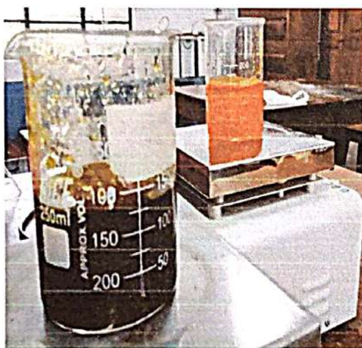
Fig 9: Before and after the addition of Co nanoparticle catalyst for the reduction of 4-Nitro phenol.
