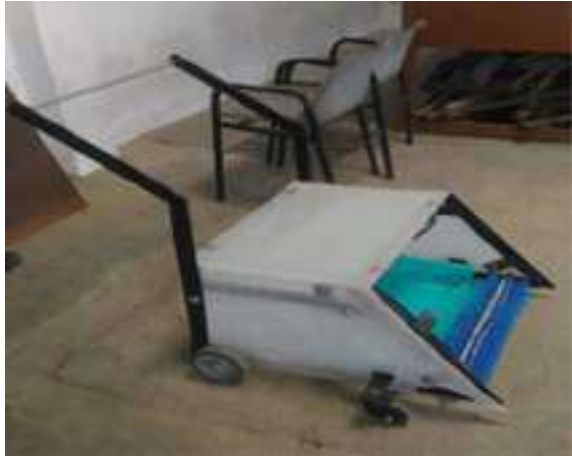
Fig. 8 Design and fabrication of manually powered path cleaner using pulley drives” international journal of engineering and advanced technology (IJEAT) Volume-9 Issue-1, October 2019 [16]
