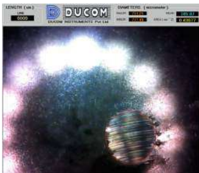
Fig. 10 Wear scar using sunflower estolide
