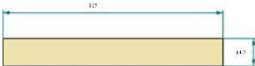
Fig. 2 Dimensions of flexural test specimen as per ASTM D790 (in mm)
