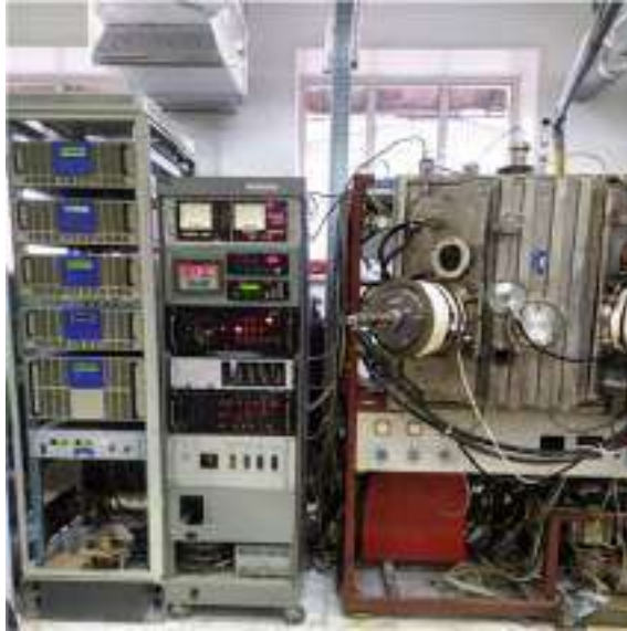
Fig. 2 The nitriding process of a disk cutter in the APP-2 ion-nitriding device of cutting tools
