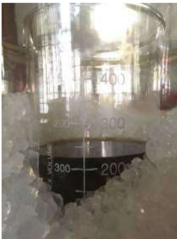
Fig. 3 Estolide ester placed between silica gel for water absorption
